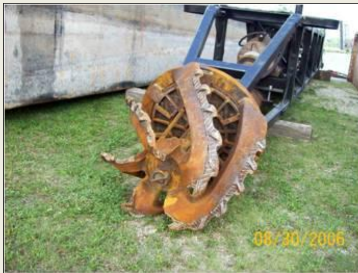
Dredge Cutter Head
